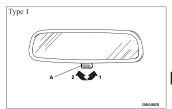
Adjust the inside mirror to maximize the view through the rear window. Make this adjustment while the day/ night knob (A) is in the daytime position (1). To reduce glare from other vehicle's headlights, switch the lever to the night position (2).
